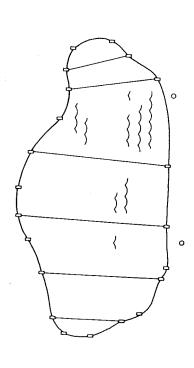
FIG. 1. Plane table map (top) showing position of a numbered shoreline stake and the base line. Distances for three shoreline points as determined by triangulation from the ends of the base line are shown. In a small lake or pond, bottom contours may be determined by sounding along a calibrated rope stretched between approximately opposite shoreline stakes (bottom).
