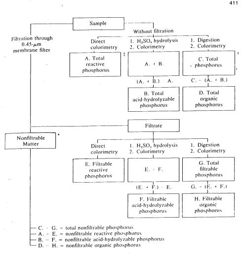
Figure 424:1. Steps for analysis of phosphate fractions.
