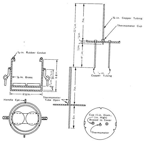
Figure 421:1. DO and BOD sampler assembly.
