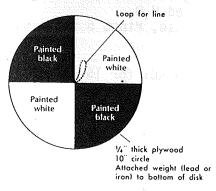
FIG. 6. The Secchi disk may be easily made from a 20-cm diameter metal or weighted wooden disk. Opposite quarters are painted gloss white and gloss black as shown. It is important that the calibrated line be attached so that the disk hangs horizontally in the water. (From Vivian, V. E.: Sourcebook for environmental education, St. Louis, 1973, The C. V. Mosby Co.)
